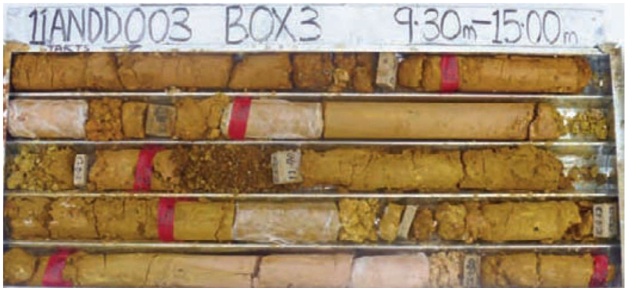
Fig. 50: Example of oxide core recovered during Phase 7. Note orange colouration.
