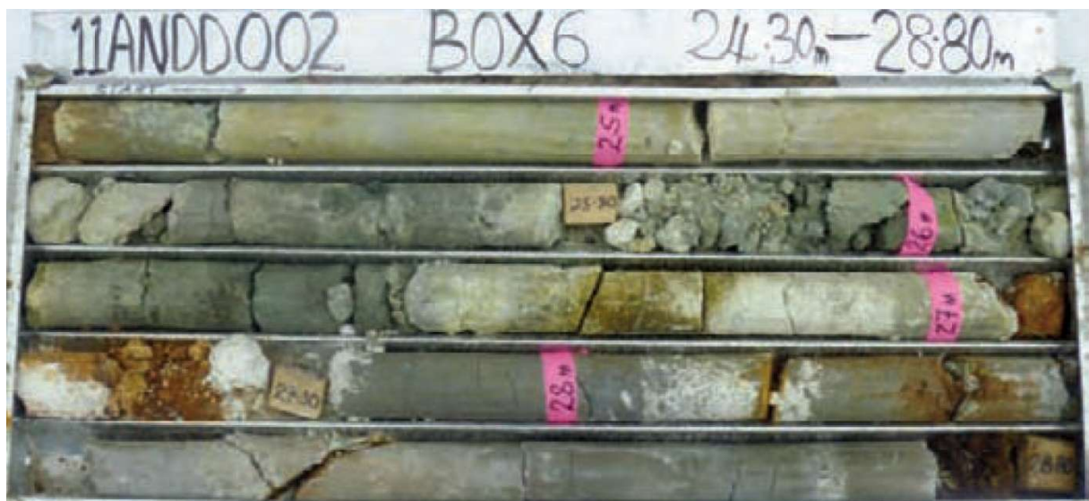
Fig. 51: Example of fresh core recovered during Phase 7. Note general greenish-grey colouration.
