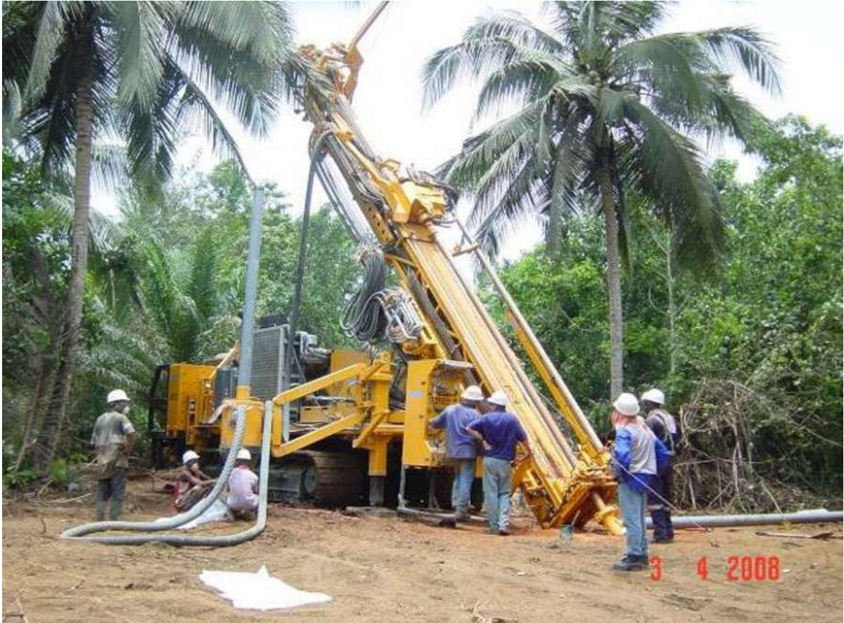
Fig. 35: Reverse circulation (RC) drilling in April 2008 at Akoko North during Phase 3
