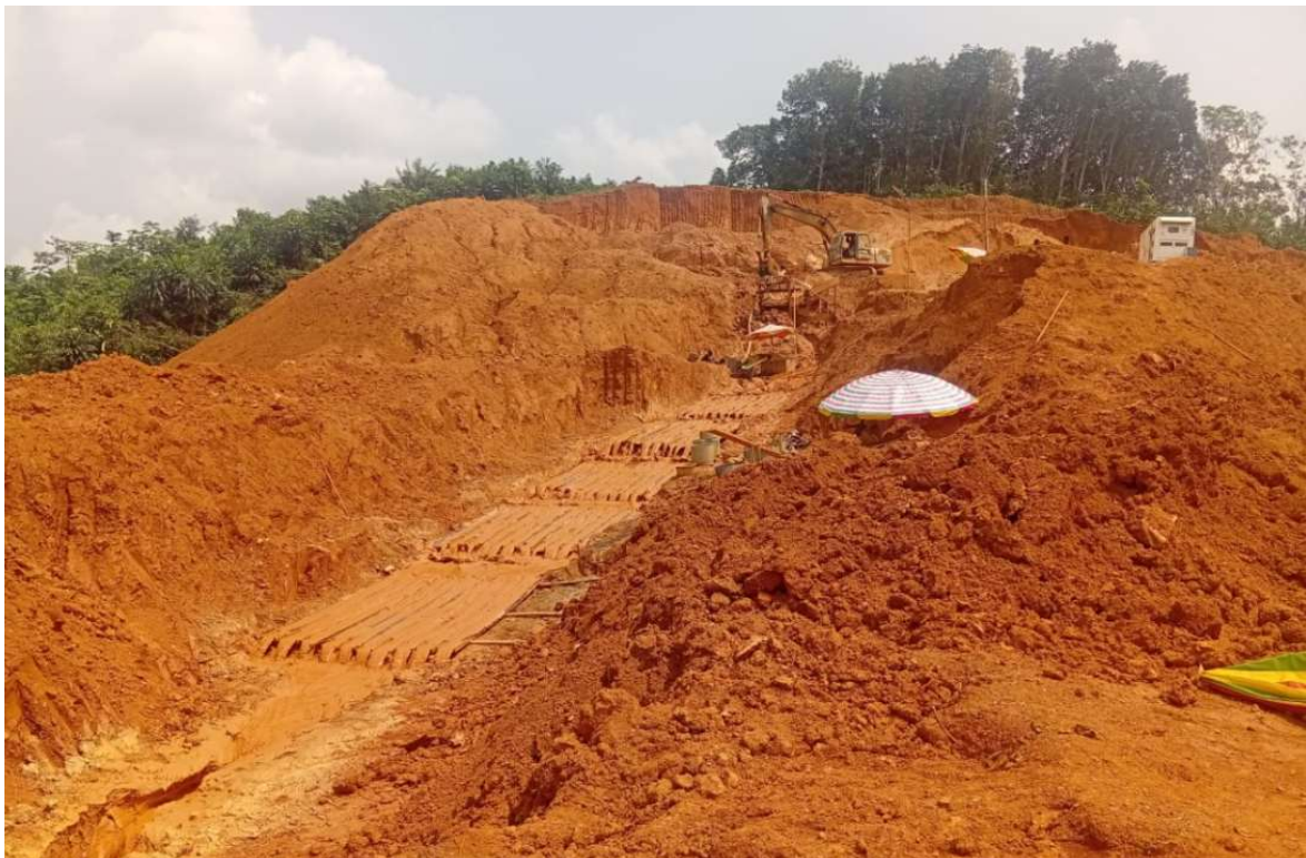
Fig. 154: Mechanized illegal mining at Akoko South, note backhoe, crusher and long flumes.
