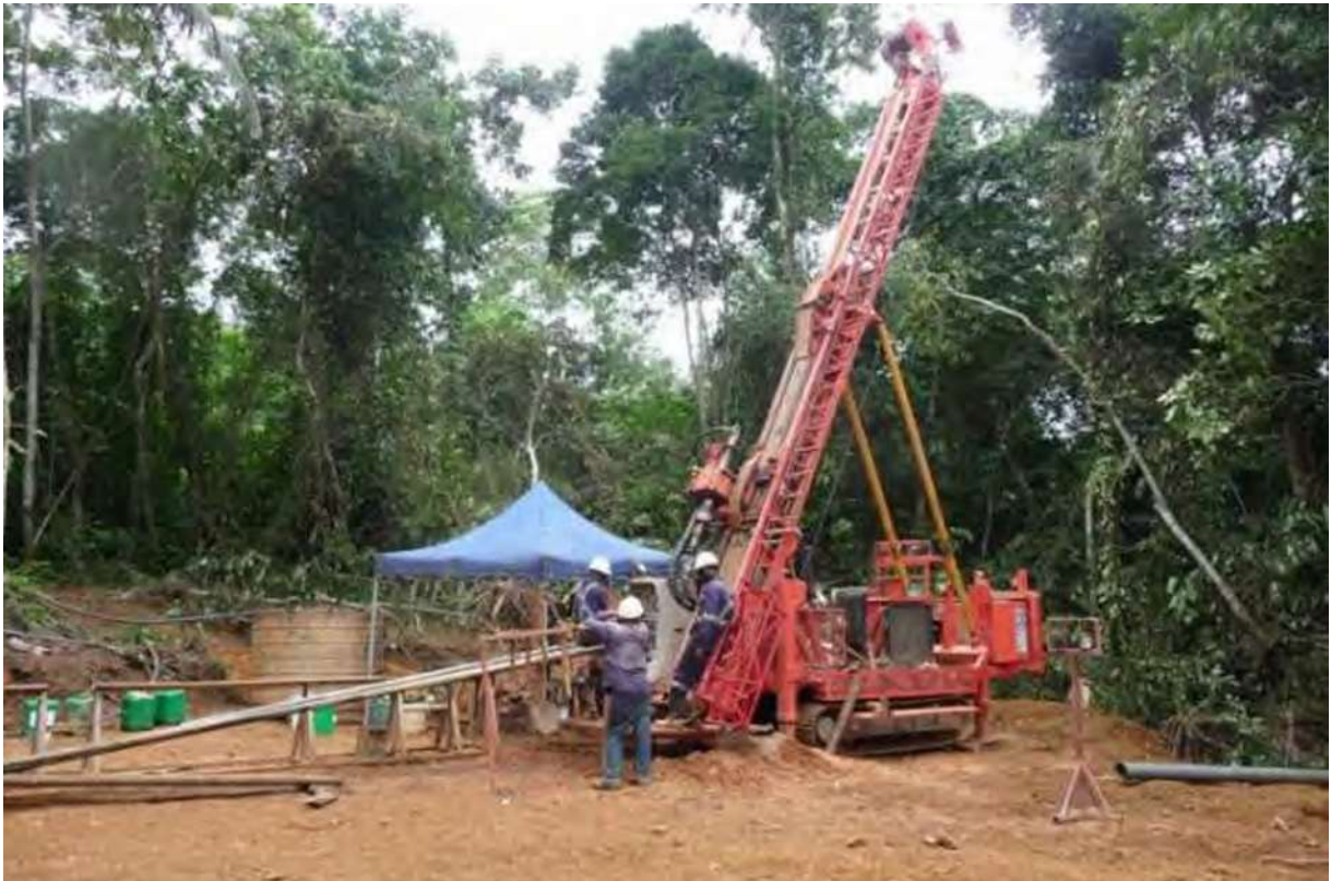
Fig. 48: Diamond rig on site at Akoko drilling 11ANDD001 in Phase 7. (Photo from Castle Minerals Ltd ASX presentation dated 2 June 2012)
