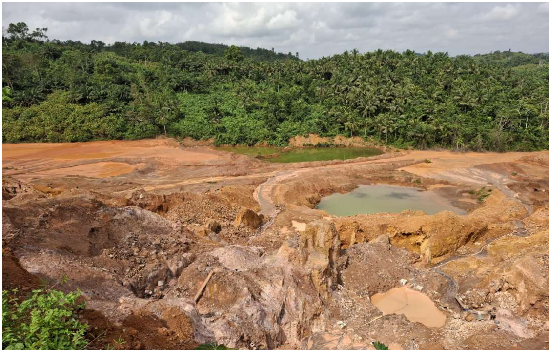
Fig. 151: Illegal workings at Akoko North showing the free digging red laterite removed down to the resistant saprock surface.
