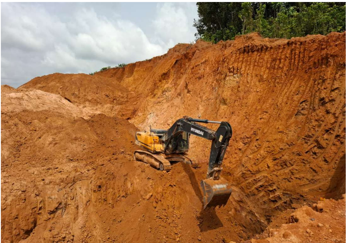
Fig. 20: Illegal mining at Akoko South – note the free digging red-orange laterite.
